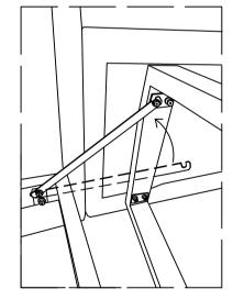
Connect the corner bench and side bench by using the fixing strap. Tighten all the bolts
